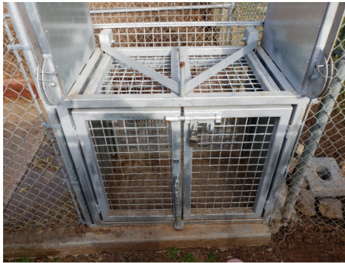
Figure 1: A version of the squeeze. The top has a pull squeeze actuator that has teeth on bar to be able to "lock" into position. The side can also be open to allow the removal of an immobilized animals.
