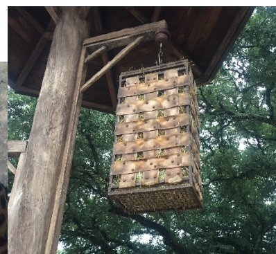
Photo 3: Final design for giraffe hay feeder
