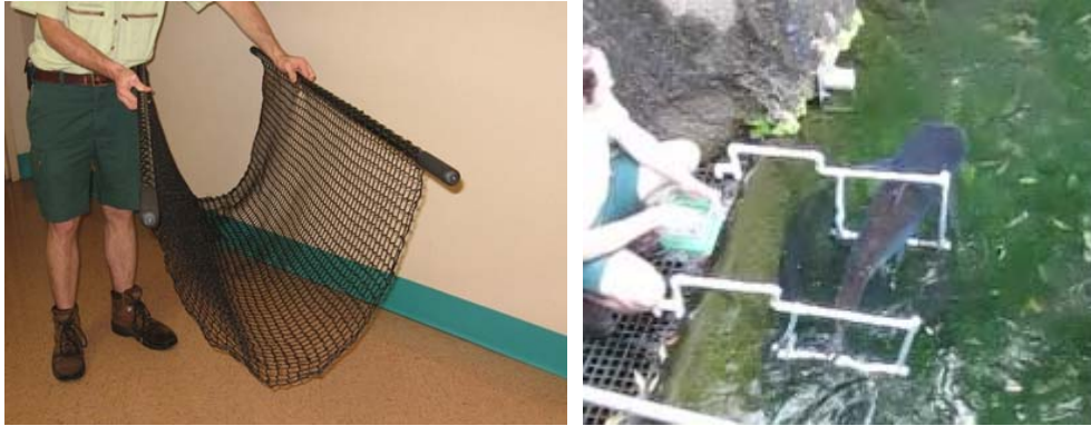
(Image 8: The cradle-net; Image 9: The pangasia swimming through two PVC squares with black, nylon, mesh on three sides.)
